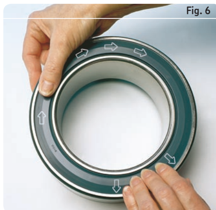
Inserting the seal in the outer ring
