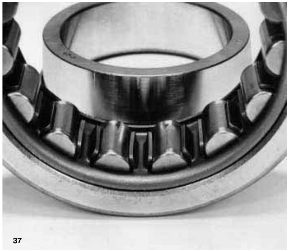
Fig 37 A cylindrical roller bearing with smear streaks in the inner ring raceway and on the rollers. The smearing has been caused by the roller assembly being entered askew without being rotated
