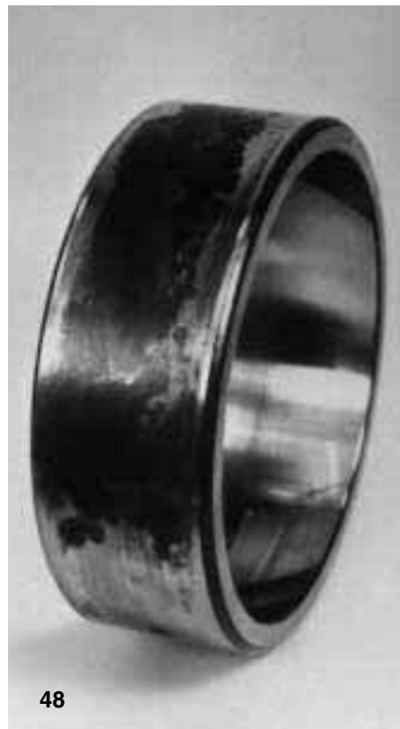
Fig 48 Fretting corrosion on the outer ring of a spherical roller bearing
