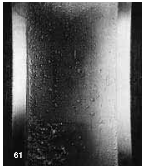
Fig 61 Cylindrical roller bearing inner ring with flaking at one side of the raceway, as a result of overloading due to misalignment
