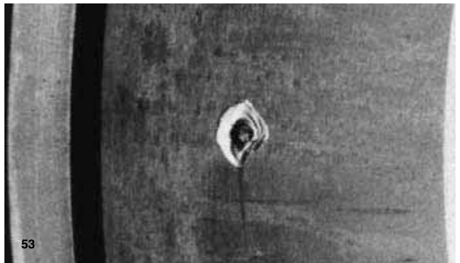
Fig 53 A railway axlebox bearing damaged by the passage of high amperage current while the bearing was not running
