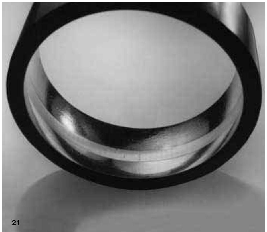
Fig 20 Cylindrical roller with mirror-like surface on account of lubricant starvation
