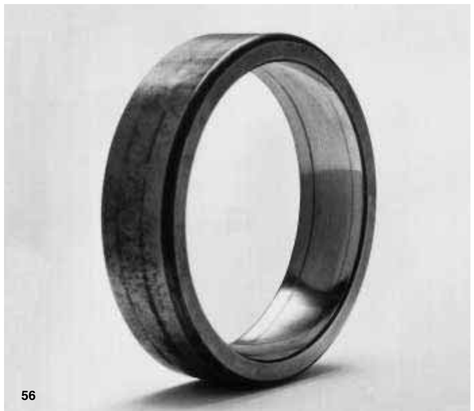
Fig 56 Outer ring of a self-aligning ball bearing that has been driven too far up its tapered seating. The bearing had only performed a few revolutions when the damage was detected. Flaking would soon have occurred if the bearing had been put into service
