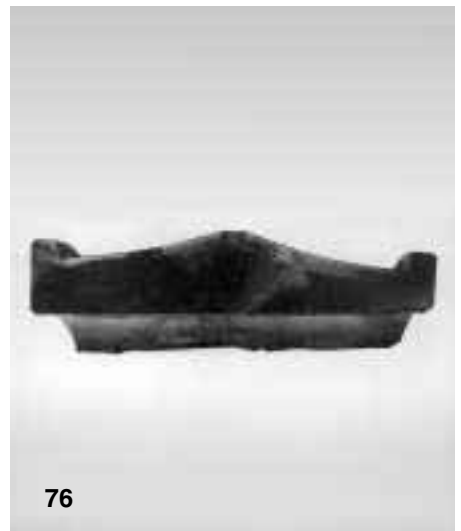
Fig 76 Fractured surface of the inner ring in fig 75
