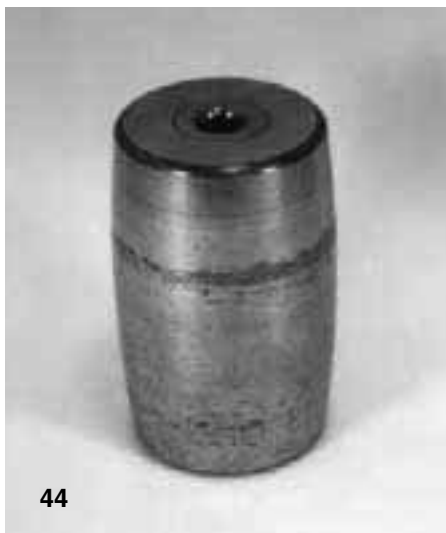
Fig 44 Surface distress in the form of a band encircling a roller from a spherical roller bearing
