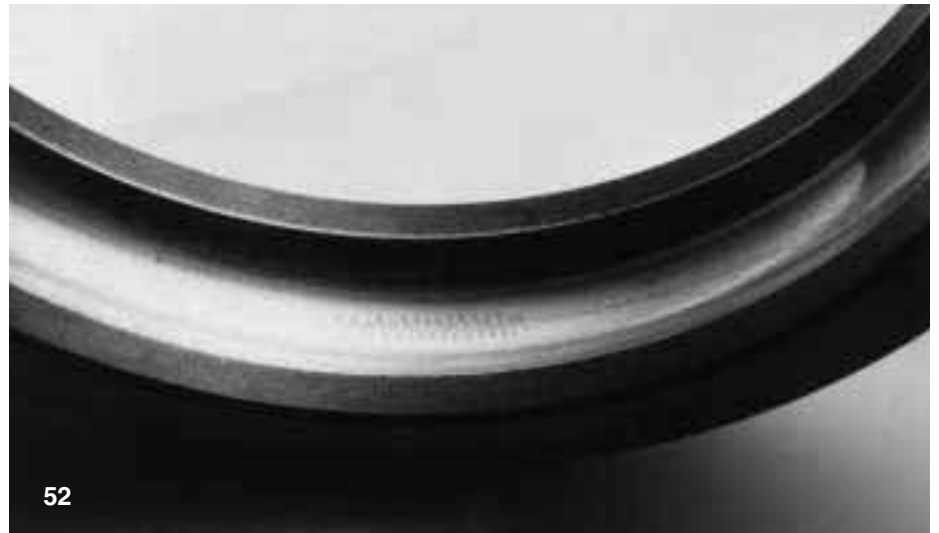
Fig 52 Deep groove ball bearing with electric current damage in zigzag pattern. It is assumed that burns of this configuration arise when the momentary passage of high amperage current is accompanied by axial vibration
