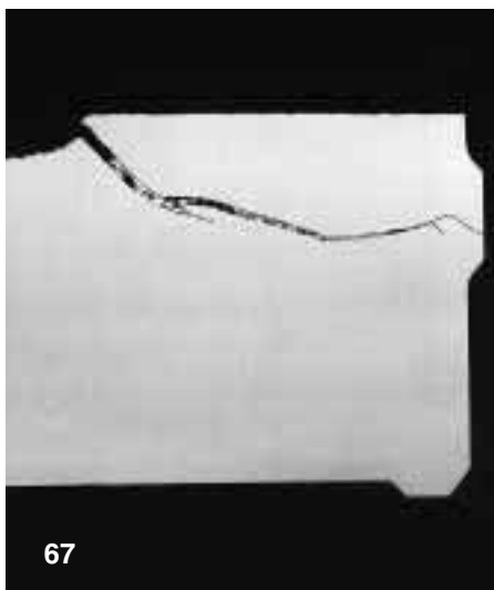
Fig 67 Cross section through the roller depicted in fig 66, showing the way in which the fatigue crack extends beneath the surface. The fully developed flaking originated in the same manner
