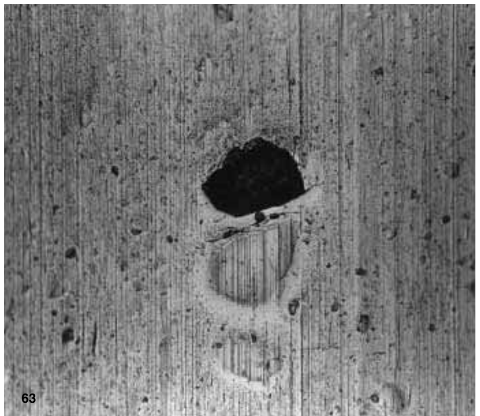
Fig 62 Various stages of flaking in the inner ring of a deep groove ball bearing. The ring has been mounted with interference fit on the shaft and blows have been directed against the outer ring, causing the mounting force to pass through the balls, which have produced the indentations
