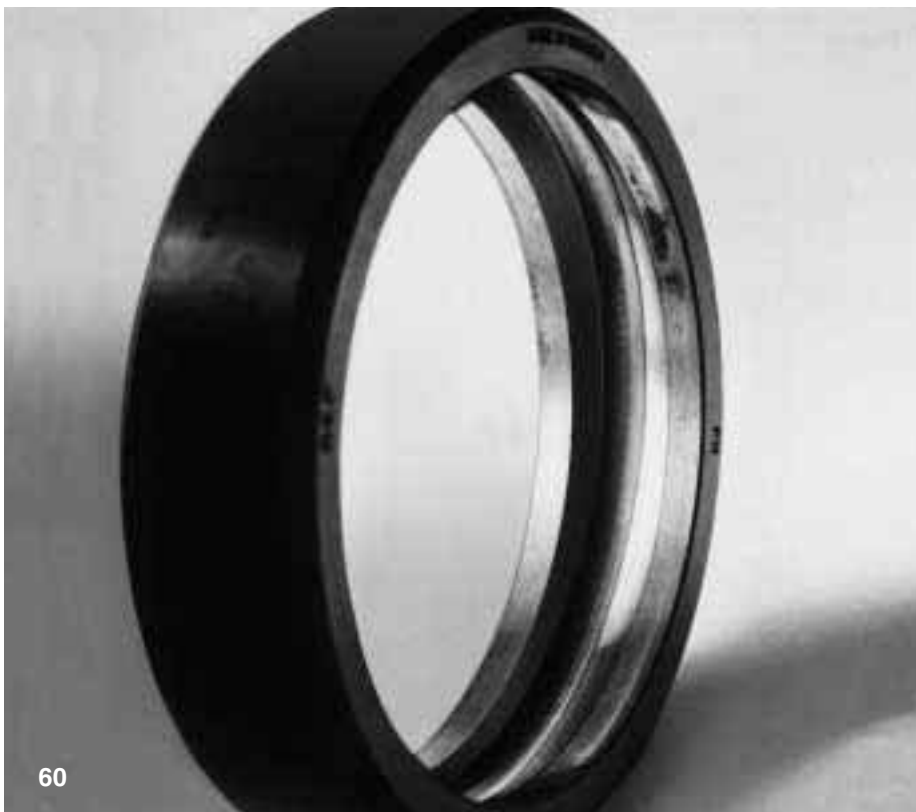
Fig 60 Deep groove ball bearing outer ring that has been out of alignment with the shaft. The ball path has an oval configuration on account of the misalignment. The result is the same as with oval compression, see page 31
