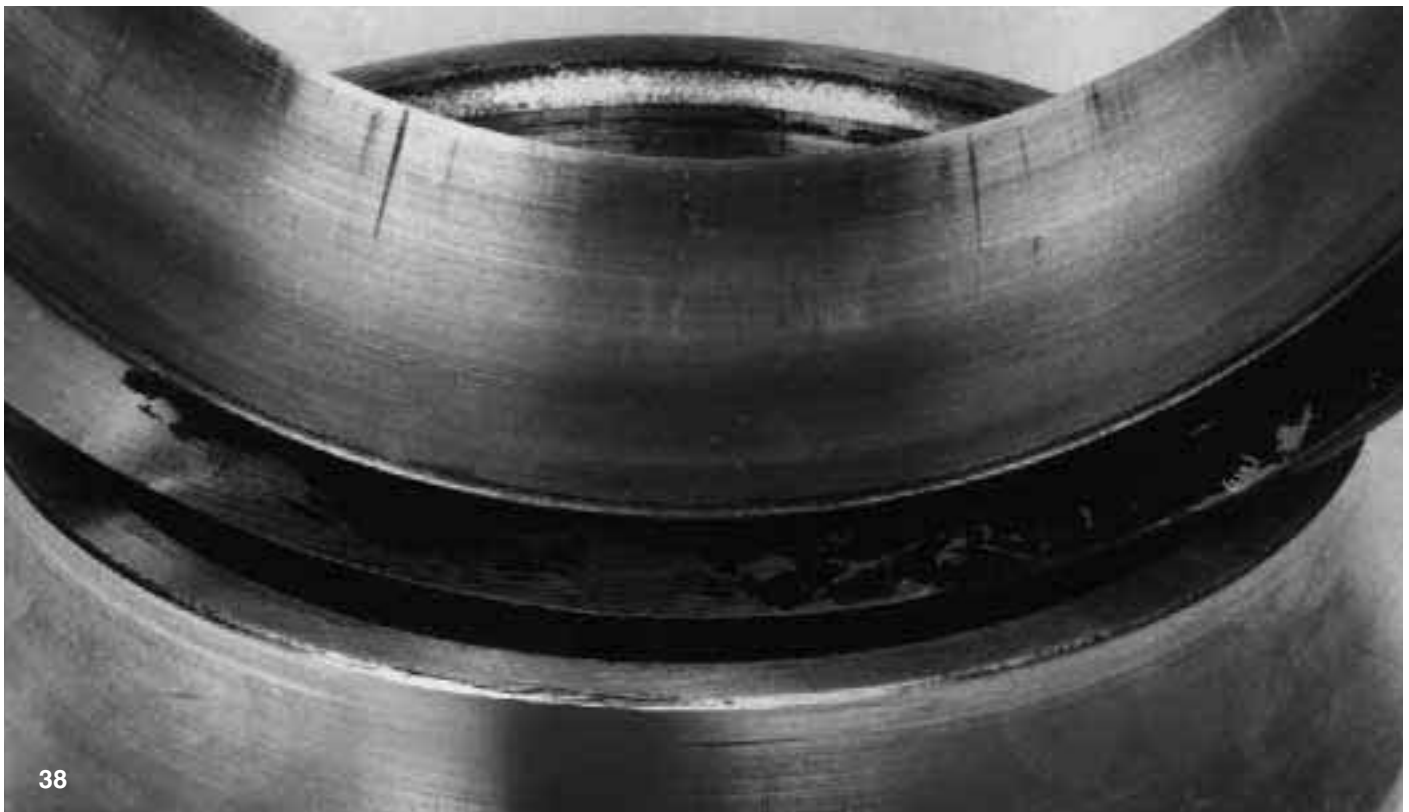
Fig 38 Outer ring raceway of a spherical roller bearing with smear streaks caused by a blow against the inner ring
