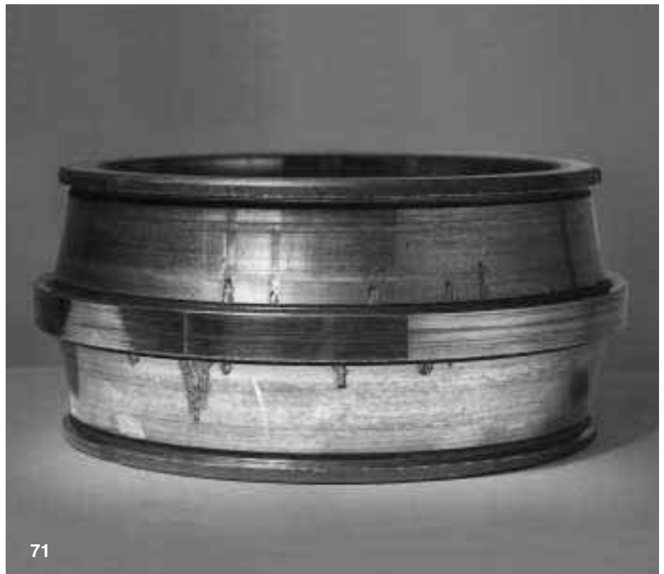
Fig 71 Flaking in both raceways of the inner ring of a spherical roller bearing. The flaking has originated from the vibration markings
