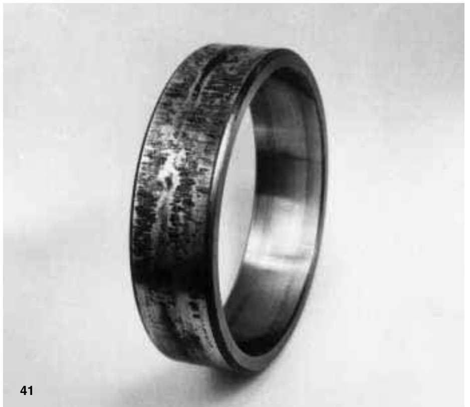
Fig 41 Smeared outside surface of a spherical roller bearing outer ring. Material transfer has occurred from housing bore to bearing ring
