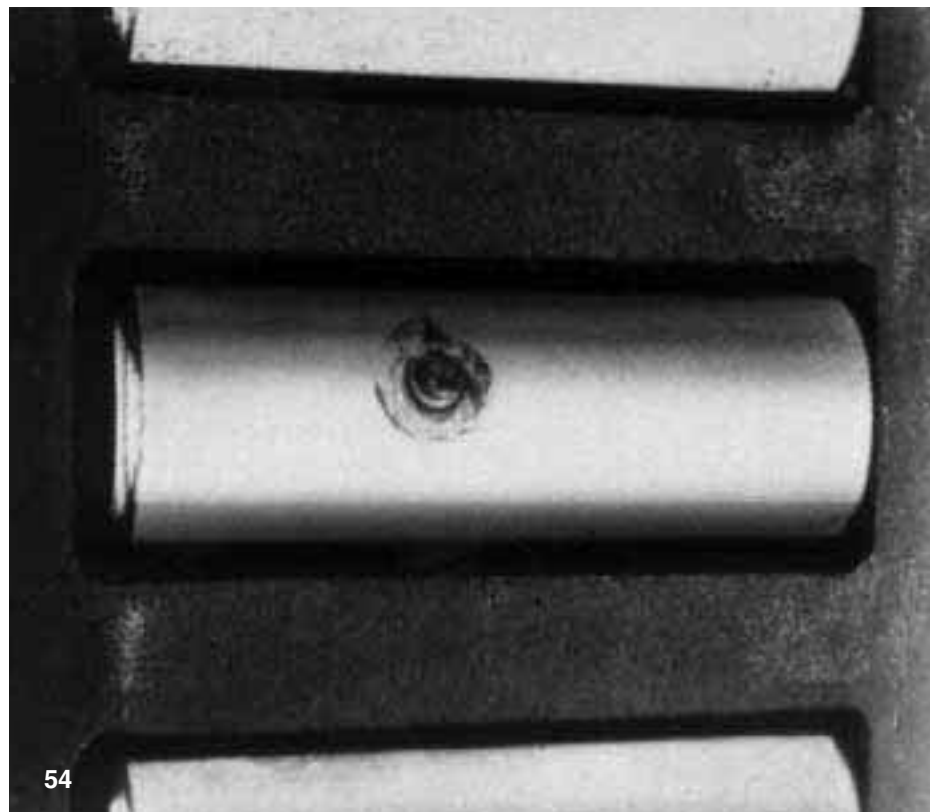
Fig 54 Roller of a railway axlebox bearing damaged by electric current (same bearing as in fig 53)
